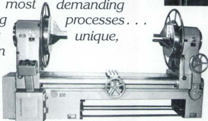
Universal glass working lathes Bores—20mm through 1200mm
