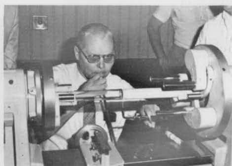
Owen Kingsbury, 38mm Mullite to Pyrex.
