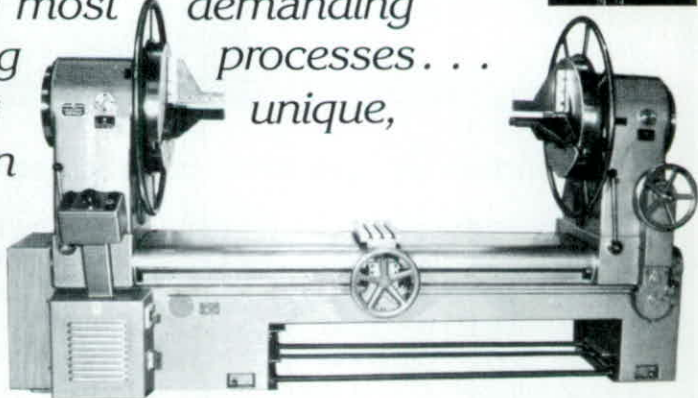
Universal glass working lathes Bores—20mm through 1200mm
