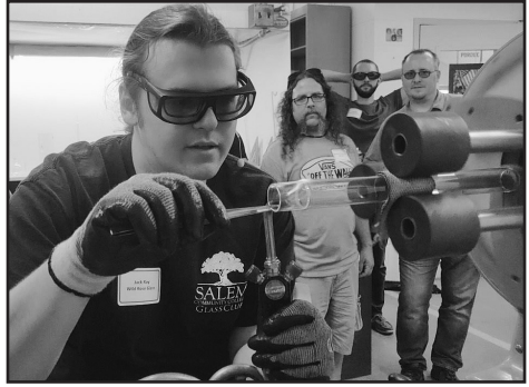
Jack Roy demonstrates fire cutting using a hand torch and tweezers
