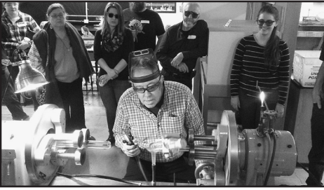
Patrick DeFlorio demonstrates making a Y-tube at the lathe
