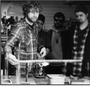
Paul Bonham walking observers through the coil wrapping process
