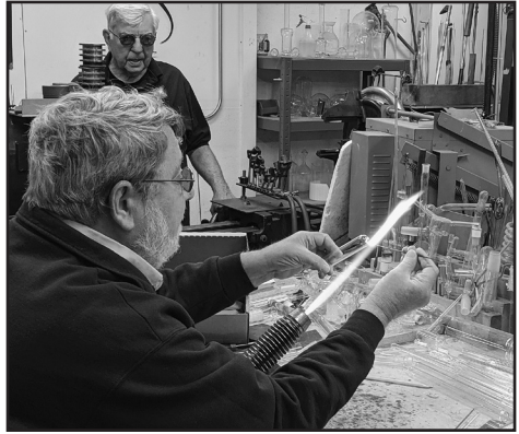
Scott Bankroff's demonstrating boring 1 mm holes into glass tubing
